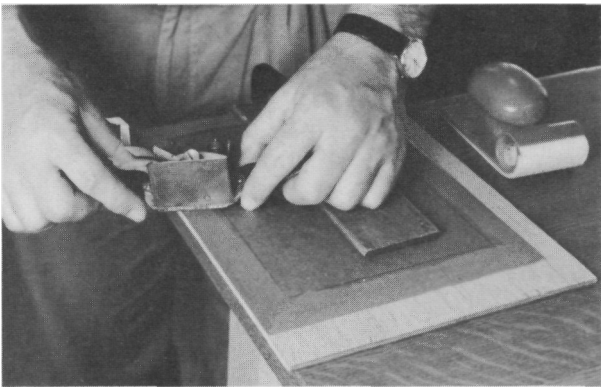
10. Board construction is the split board type. The top board is cushioned on all four edges.
