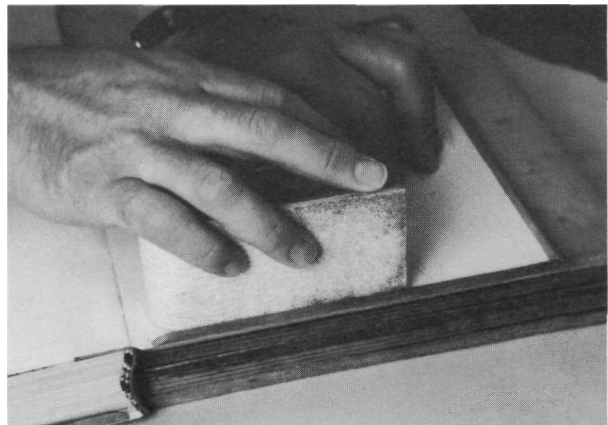
14. As there is no rounding and backing with this method, there is no joint to give support to the text-block. Therefore a yapp support edge (in this case a wooden beading) is attached to the squares on each board. This locates over the text-block when the boards are closed and ensures that the text-block does not sag when the book is standing.
