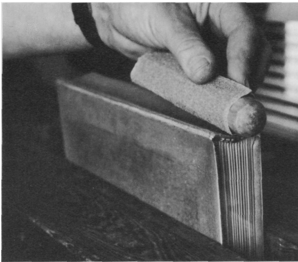
16. The spine linings are sanded off at an angle at head and tail to accommodate the thickness of the turn-ins, giving a smooth spine.
